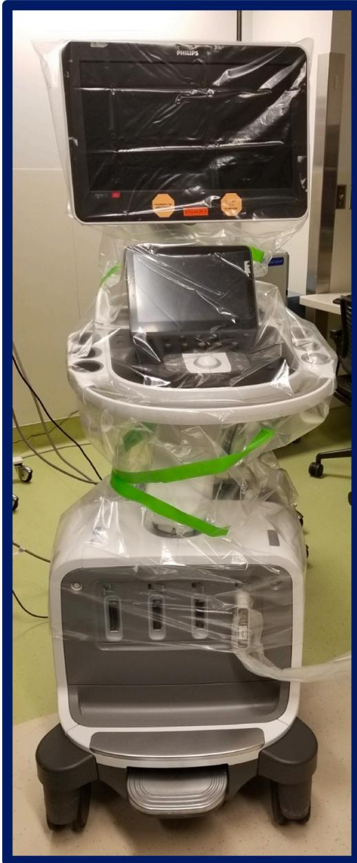
Figure 2. Ultrasound system with transesophageal echocardiography capabilities is shown with a plastic cover. The screen, touchable parts and the transducer ports are covered by the disposable plastic cover.
